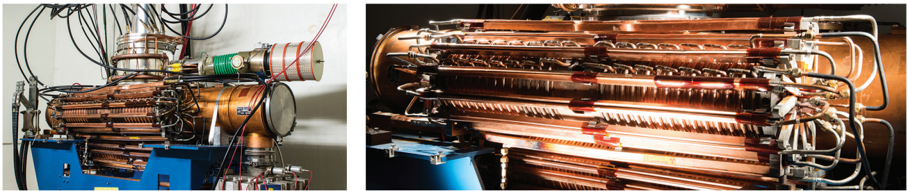
FIGURE 2: At left, a photograph of a copper ferrite-tuned RF cavity from FNAL's Booster synchrotron. At right, a ferrite tuner.
