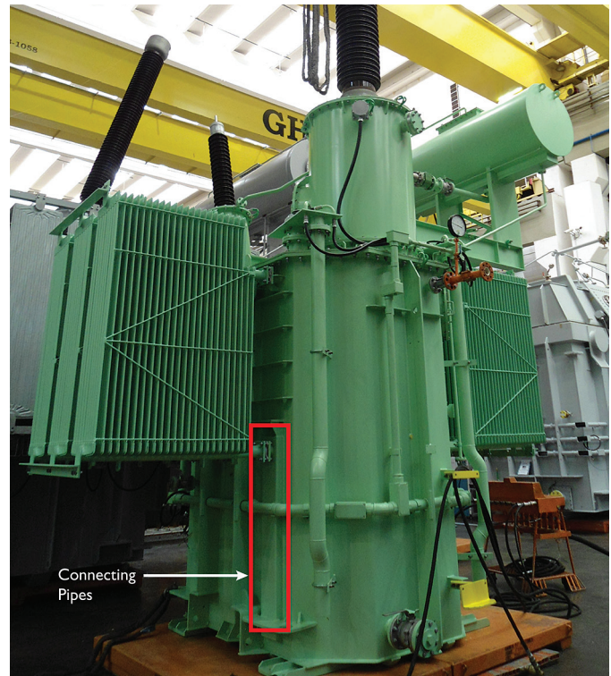
FIGURE 1: Shunt reactor. In the original design of the oil circuit the radiator is connected to the tank by pipes enclosed in rectangular boxes welded to the exterior of the reactor.
