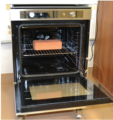
FIGURE 1: Left: Whirlpool's Minerva oven set up for the "brick test." Right: The meshed geometry.
