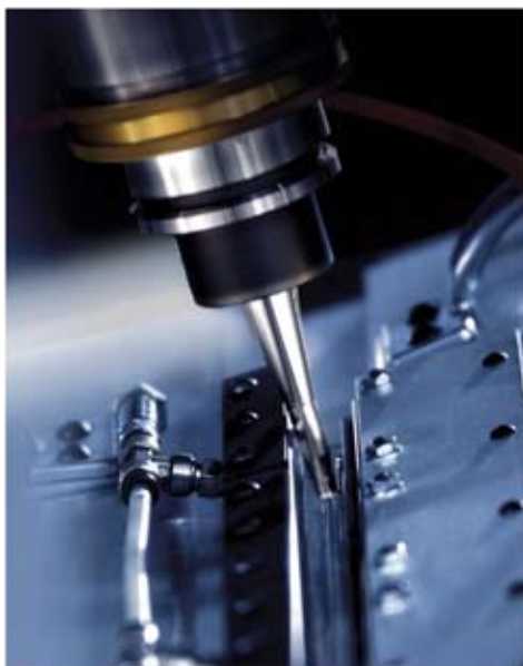
Figure 1: In Friction Stir Welding, a shoulder sits on the metal surfaces and creates heat through friction, while a pin stirs the plasticized-heated materials to create the weld. (photo courtesy of Eclipse Aviation, Albuquerque, New Mexico)
