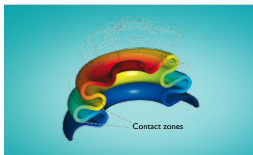
Figure 2: The collapsed rubber seal and the zones of contact.
