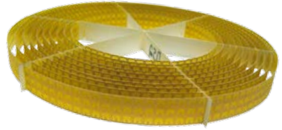
Figure 3: The 2D cloaking structure where the electromagnetic radiation is limited to the x-y plane. An object located in the center of this structure is almost invisible to microwave radiation in a narrow range of frequencies. (photo: Smith, Schurig, Pendry, and Cummer, Science )
