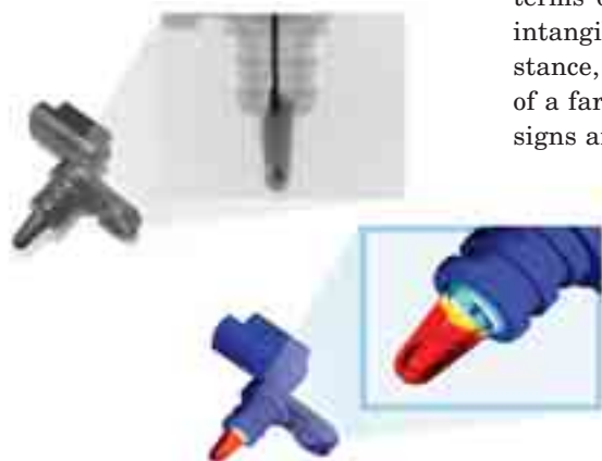
Figure 2: A photograph and X-ray picture of a temperature sensor and a model plot of temperature distribution over the whole of the sensor and on the sensing element inside the cap.
