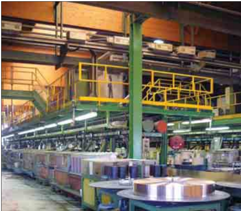
Figure 1: Factory floor with a series of reel-to-reel electroplating units. Reels of solid or stamped metal plates are passed through the electroplating units, and metal is deposited over the whole or sections of the tape according to the application of electric current and the placement of shields.
