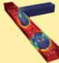
Model of droplet breakup created with the Level Set method.
