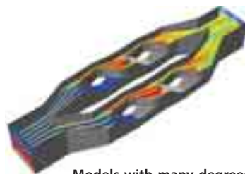
Models with many degrees of freedom, such as this static mixer, benefit greatly from multicore parallel processing.
