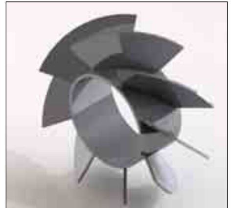
Figure 2: Geometry of the axial swirler.
