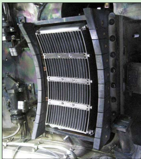
Lower hybrid grill antenna as seen from inside of the Alcator C-Mod vessel. The arrays of open-ended waveguides are phased so to launch the waves preferentially in one toroidal direction, so accelerate electrons and ultimately drive current inside of the plasma.
