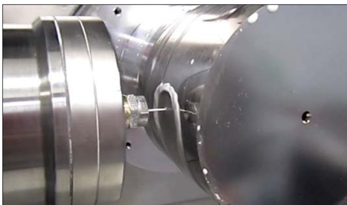
Figure 1. Fluid jet polishing of an aspheric die for thin X-Ray mirror replication. See the video at www.comsol.com/video/337/ .
