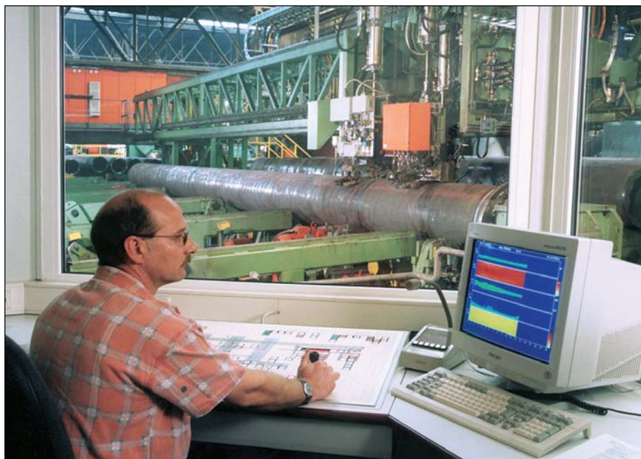
Figure 2. An inspection in operation: the yoke is embedded in plastic behind the orange box and as the pipe is rotating, the box moves along the pipe, 1 mm above the surface.
