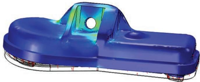
**FIGURE 1.** Top: A Hi-Speed Snap-In Tire Pressure Monitoring Sensor (TPMS) used to monitor tire pressure and send measurement info. Bottom: 10x amplification of stress and deformation on the transmitter housing as a result of centrifugal loading produced by the wheel's rotation.
