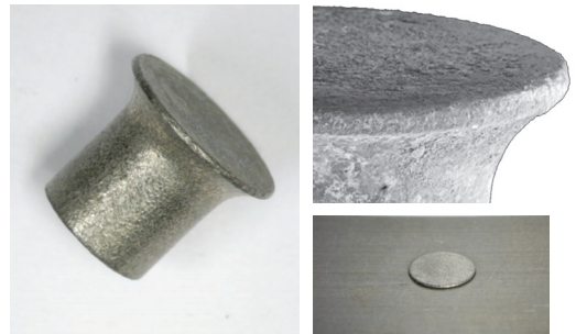
FIGURE 1. Left: Clean rivet. Top right: Rivet showing magnesium hydroxide deposit (white growth) due to corrosion. Bottom right: Magnification of a rivet in a test sheet.
