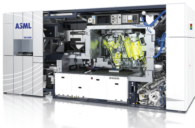
FIGURE 2. The ASML® TWINSKAN® NXE:3350B production-ready EUV system produces 125 computer wafers per hour using 13.5 nm wavelength light. It must keep a perfect vacuum while moving wafers at high speeds and loads, maintaining distortions to less than 1 nm.
