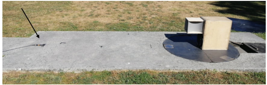
FIGURE 3 Outdoor measurement setup for a typical acoustic loss measurement. Arrow indicates position of microphone.
