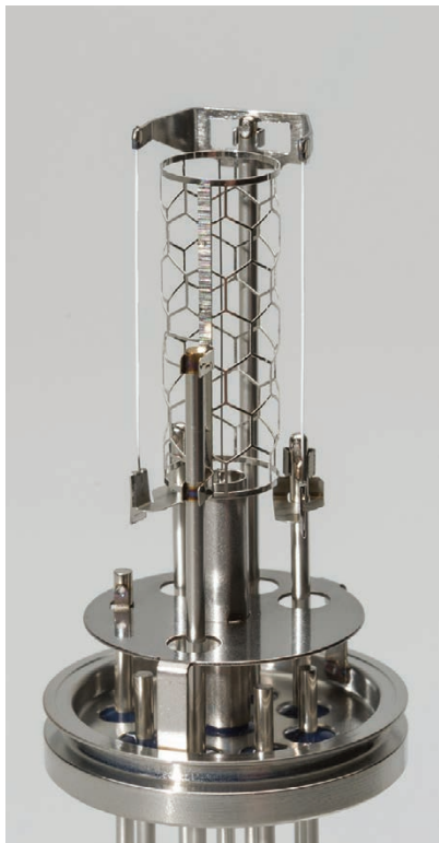
FIGURE 2 A Bayard–Alpert hot-filament ionization gauge. Image provided by INFICON.
