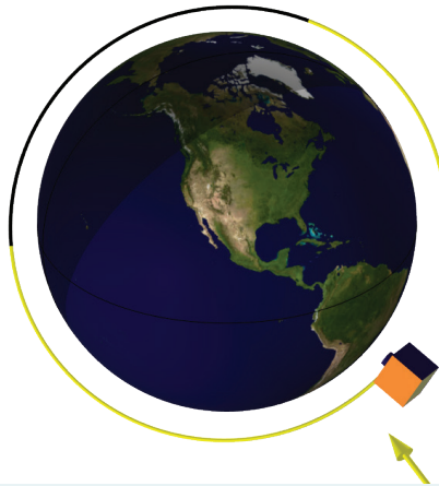
FIGURE 3 A visualization of a satellite in orbit, showing the position and orientation relative to the Sun and Earth as well as the irradiation onto the satellite's exposed faces. Earth image credit: Visible Earth and NASA.
