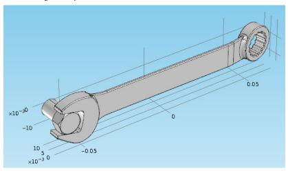
The bolt's fixed constraint is at the cross section shown below. A load is applied at the box end of the combination wrench.
