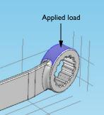
Here, assume that there is perfect contact between the wrench and the bolt. A possible extension is to apply a contact condition between the wrench and the bolt where the friction and the contact pressure determines the position of the contact surface.
